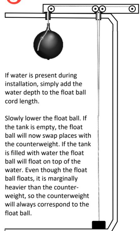
If water is present during installation, simply add the water depth to the float ball cord length.
