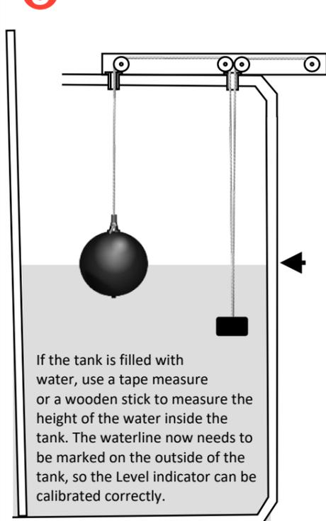
If the tank is filled with water, use a tape measure or a wooden stick to measure the height of the water inside the tank. The waterline now needs to be marked on the outside of the tank, so the Level indicator can be calibrated correctly.
