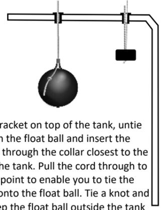
With the bracket on top of the tank, untie the knot on the float ball and insert the cord down through the collar closest to the center of the tank. Pull the cord through to the access point to enable you to tie the cord back onto the float ball. Tie a knot and fasten. Keep the float ball outside the tank
