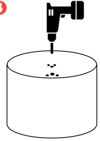
You should end up with 2 large holes (25/64" or 10mm) and 4 small marks in the top of your tank:
