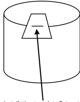
Lay the installation template flat on top of the tank. Tape down the corners, if necessary, to secure the template. Line up the template until the edge of the tank marking and the edge of the tank line up. Drill (2) 25/64" or 10mm holes for the black plastic cord collars, starting with increasingly larger pilot holes. A 3/8" hole (slightly enlarged) will also work.
