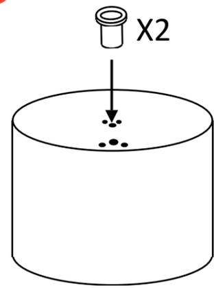
Insert the 2 black plastic cord protection collars into the holes. Please note that these collars should fit tightly into the tank, so they may need to be tapped in gently using a hammer or a mallet.
