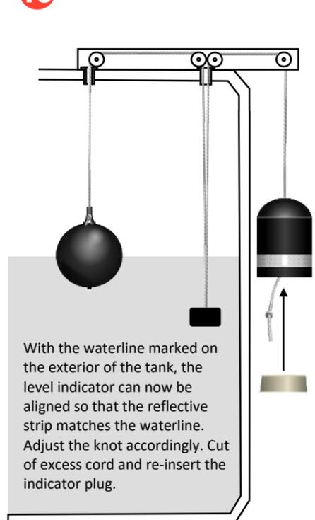
With the waterline marked on the exterior of the tank, the level indicator can now be aligned so that the reflective strip matches the waterline. Adjust the knot accordingly. Cut of excess cord and re-insert the indicator plug.
