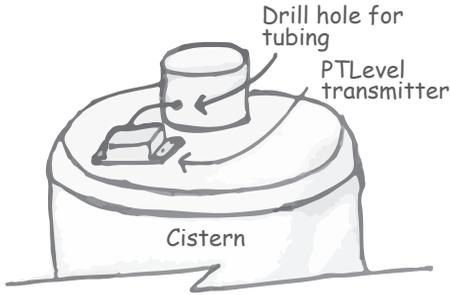
The main idea is to mount the device outside of the tank.
