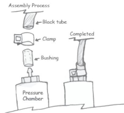
**Note:** Make sure all tubing connections are setup and sealed properly or the PTLevel will not read accurately.
