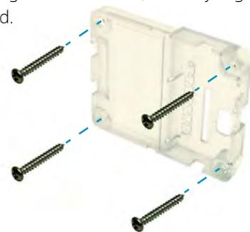
Screw the backplate onto the surface.
