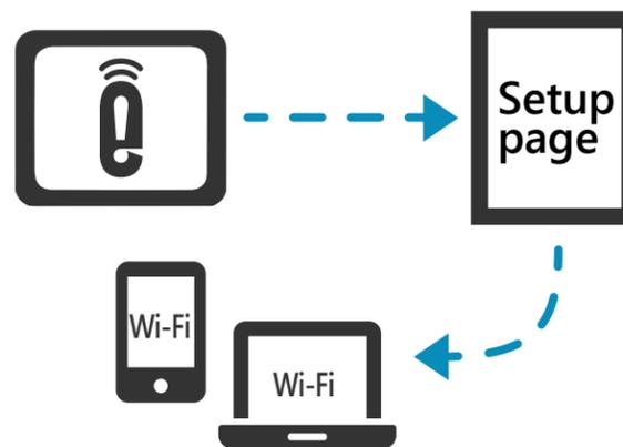
The Elertus Wi-Fi network cannot provide an internet connection, but will provide access to the Elertus setup web page.
