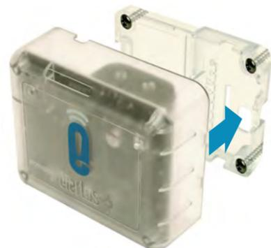
Finally, attach the Elertus Sensor to the backplate and you are done.
