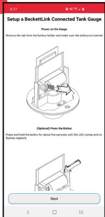
5 Be sure the plastic tab has been removed from the battery holder and that the battery is seated firmly in the holder. The green LED next to the battery holder should flash once every 16 seconds in discovery mode. Optional: press and hold button next to the battery folder for 5 seconds until the LED comes on and flashes regularly. If the LED comes on solid and stays on, the gauge is already paired and must be unpaired before starting the process. (See Un-pairing)
