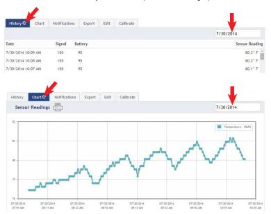
**Note:** To change the date range of the viewable information, click on the date range box at the top right of the sensor detail panel.
